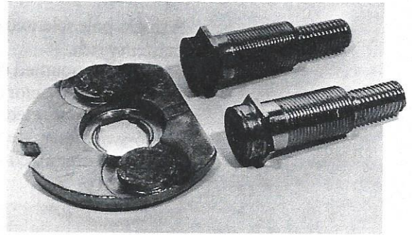
Contact wear results in control system failure.
